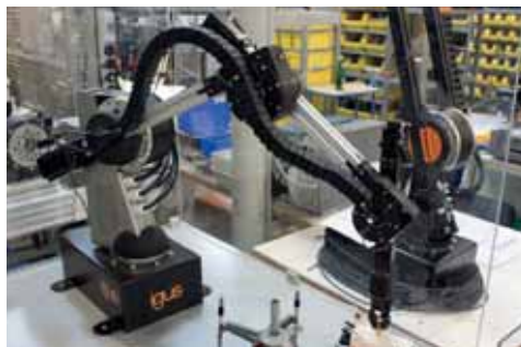
售货系统应用 - 5轴机械臂RL-DQ-RBT-5532S-AC 和3指机械爪 Trade fair machine RL-DQ-RBT-5532S-AC with 5 DOF and 3-finger gripper (igus® GmbH)
