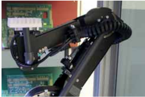
用于PCB检测的robolink® D 机械臂 robolink® D for checking printed circuit boards (4Stars Engineering Systems GmbH)
