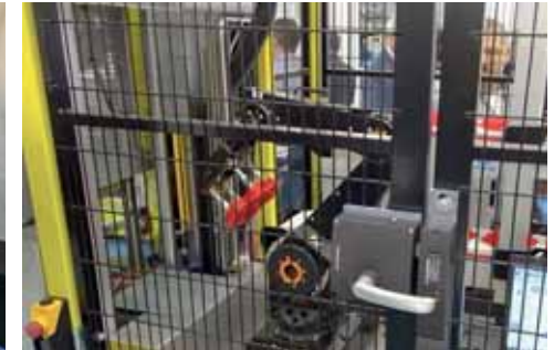
4轴的robolink® D 用于自动化注塑 Injection-moulding process with automated handling thanks to robolink® D with 4 DOF (Dr. BOY GmbH & Co. KG)
