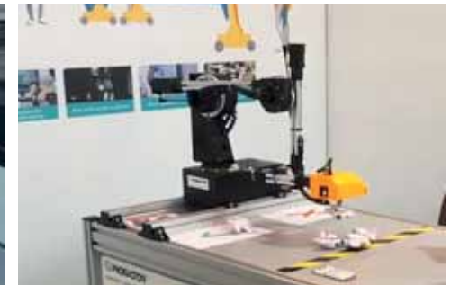
用于分拣的RL-DQ-5532S和 CPR 控制系统 Measuring machine with RL-DQ-RBT-5532S and CPR control system for sorting good from bad parts (PROFACTOR GmbH)
