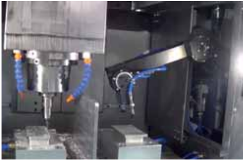
机床上带吸盘的robolink® D robolink® D – Suction arm in a machine tool (igus® GmbH)
