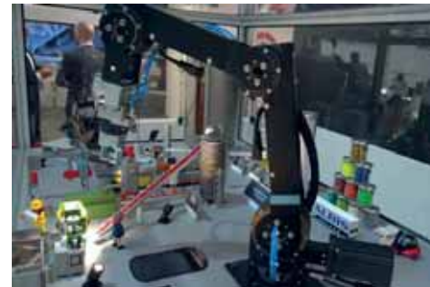
4轴的robolink® D 用于工厂自动化 robolink® D with 4 DOF as manipulator in demo factory (ALBIS PLASTIC GmbH)
