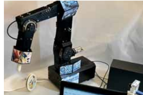
视觉控制的5轴机械臂 Camera-based control of a sensorless RL-D arm with 5 DOF (RoVi Robot Vision, TU Munich, LMT)
